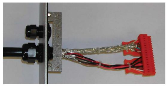
It is very important that the outer cable shield is connected to the rear plate at the cable entry and that the shield around the Ethernet pairs are run to the orange terminal block as shown in the picture.
